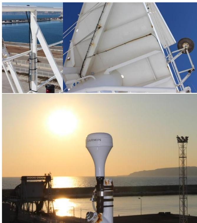
**Figure 11:** View of air inlet (top left and right) and GPS sensor (bottom).
