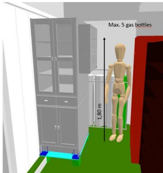
Figure 4: Setup of RINGO-ATC-SOOP System in the crews firefighting preparation room as approved by Chief of SOOP TAVASTLAND.
