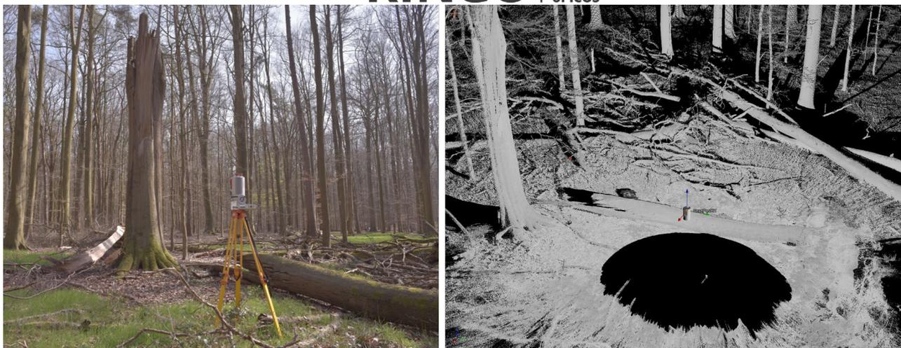
Figure 1: Laser scanner in operation in a beech forest with considerable amounts of standing and lying deadwood. (left) A tripod is used to stabilise the scanner and to gain a higher point-of-view, and (right) the resulting 3D scan, coloured on reflectance.
