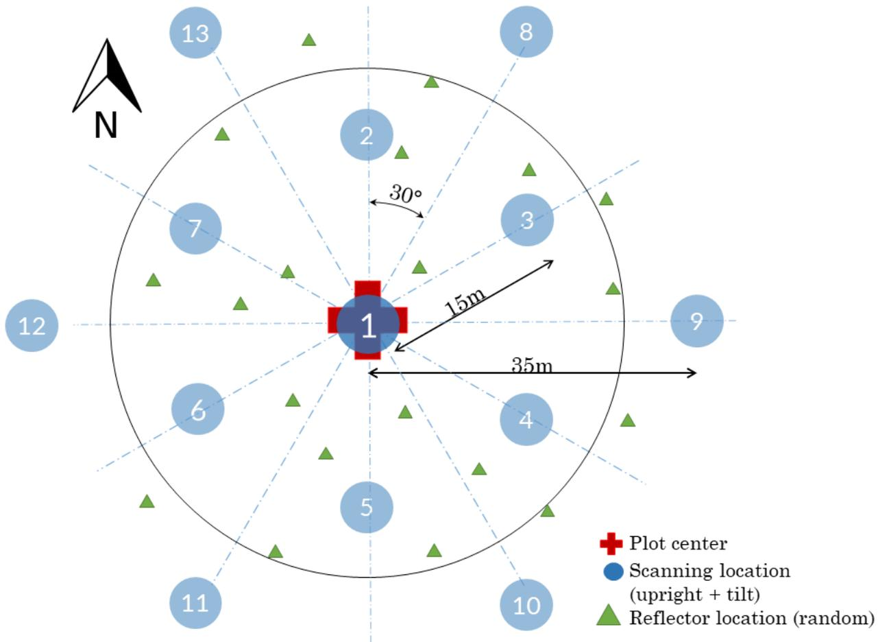
Figure 2: Data-acquisition for geometrical modelling of above-ground biomass with terrestrial laser scanning: scanning pattern in the 25m radius ICOS continuous measurement plots. The scanning chain order is indicated with numbers on the scanning locations. First, the centre location is scanned. Subsequently, starting North, the other locations are scanned in two circles around the centre.
