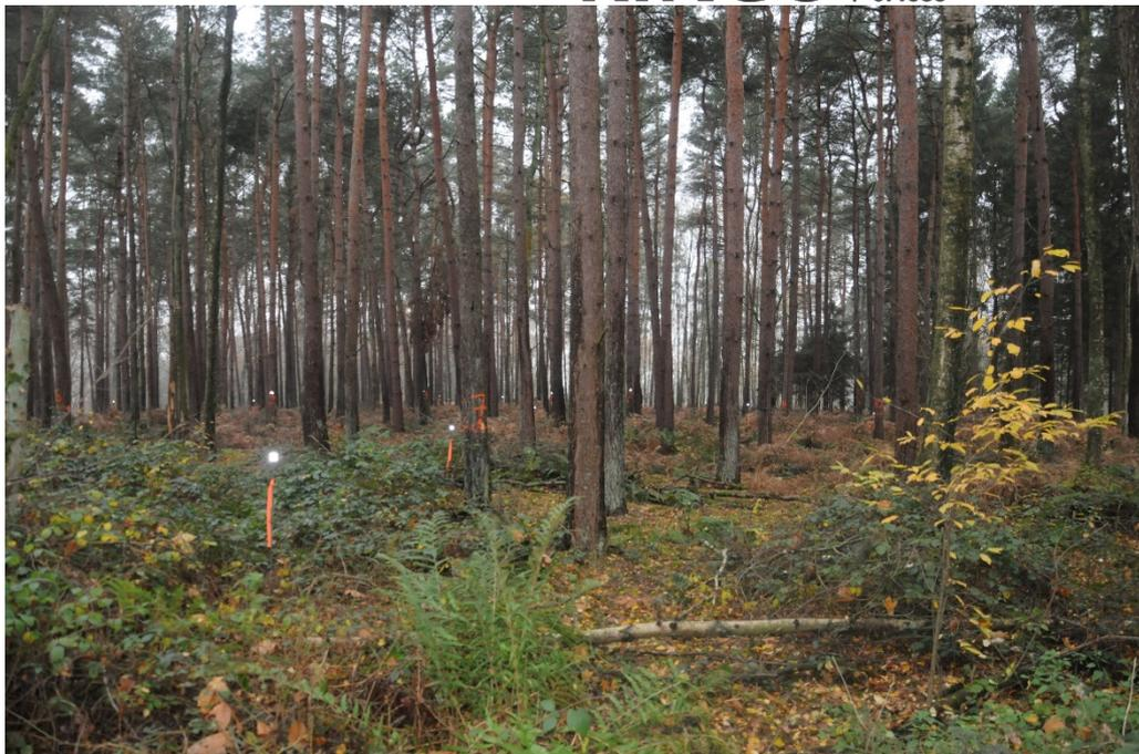
*Figure 3: Retro-reflective target positioning: targets are put on poles, firmly planted in the forest soil and at ~1.5m from trees for improved visibility. Photo-degradable forest tape (orange) helps to find all the poles back after scanning.*
