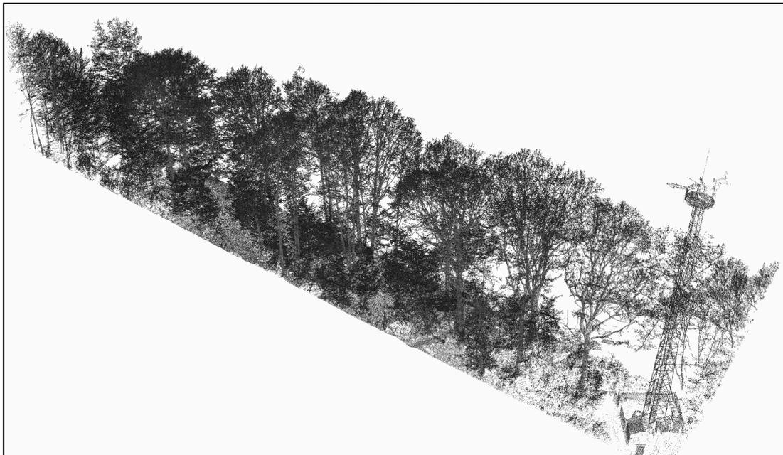
Figure 5: A slice from a coregistered pointcloud at the FR-FON site in Barbeau, combining 26 scans from 13 positions. The scanning grid is designed to capture full 3D pointclouds inside the CPs. Vegetation and measurement masts outside the CP are also partly covered. However, for volume reconstructions they are not sufficiently complete.
