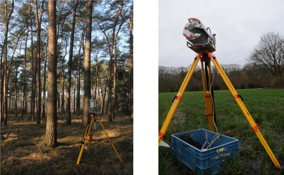
Figure 4: Riegl VZ-400 time-of-flight terrestrial laser scanner at work. An upright scan can rotate 360° with a 100° viewing angle (left). Adding an tilted scan (right), will produce a view above the scanner. If the two are combined from the same scanning position, a full hemispherical view is produced.
