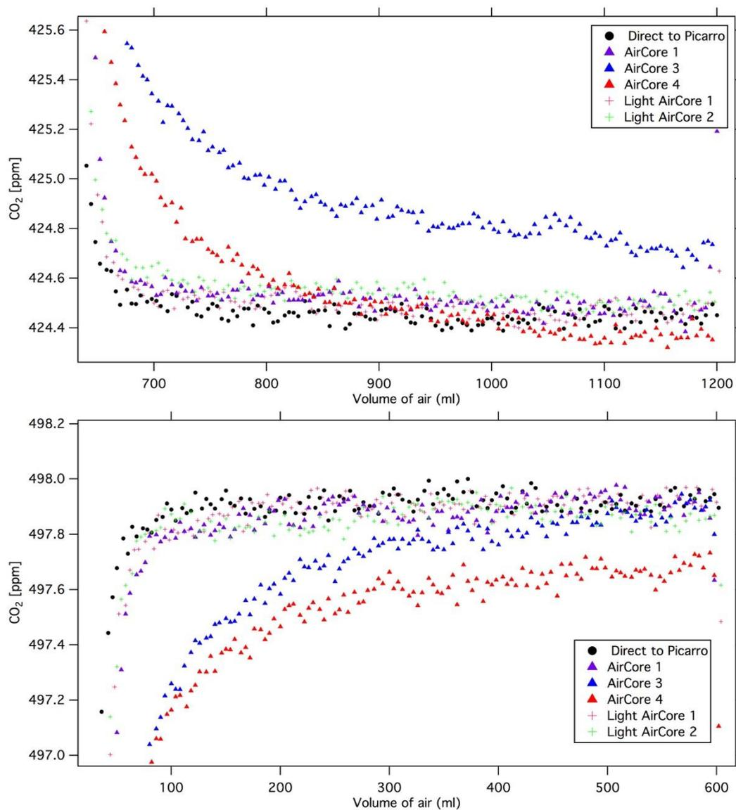
Figure 8. Slug test results of CO<sub>2</sub> as a function of the volume of air (ml) flushed since the start of the transition from high to low mole fractions (top) and from low to high mole fractions (bottom) for five AirCores.
