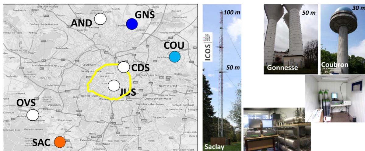
Figure 1: Left: map of the monitoring stations around Paris. Right: pictures of the sites and analyzers.
