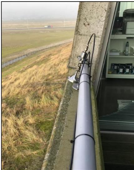
Figure 5: The filtering funnel on the air inlet
